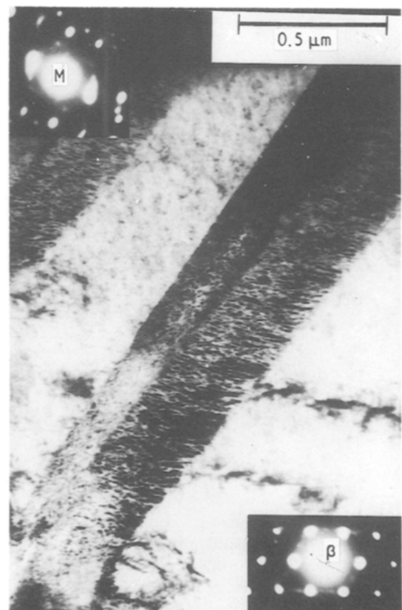
Figure 3 Martensite plate morphology under 1.2 MV TEM at 243 K.
