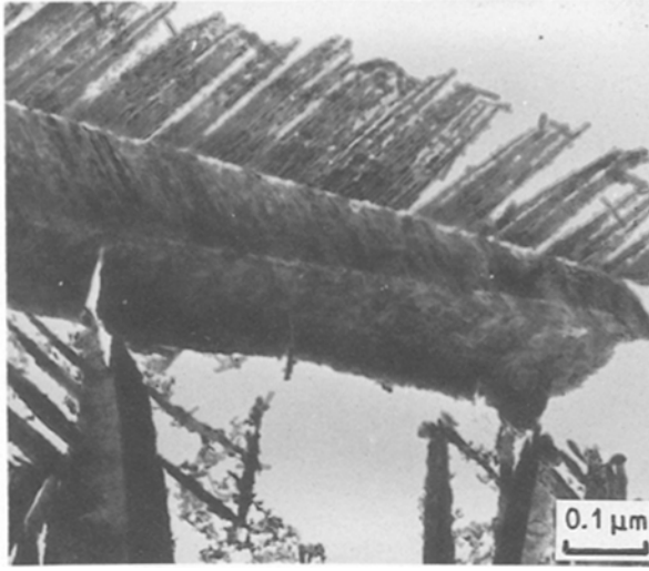
Figure 9 Martensites consisting of tiny packets.
